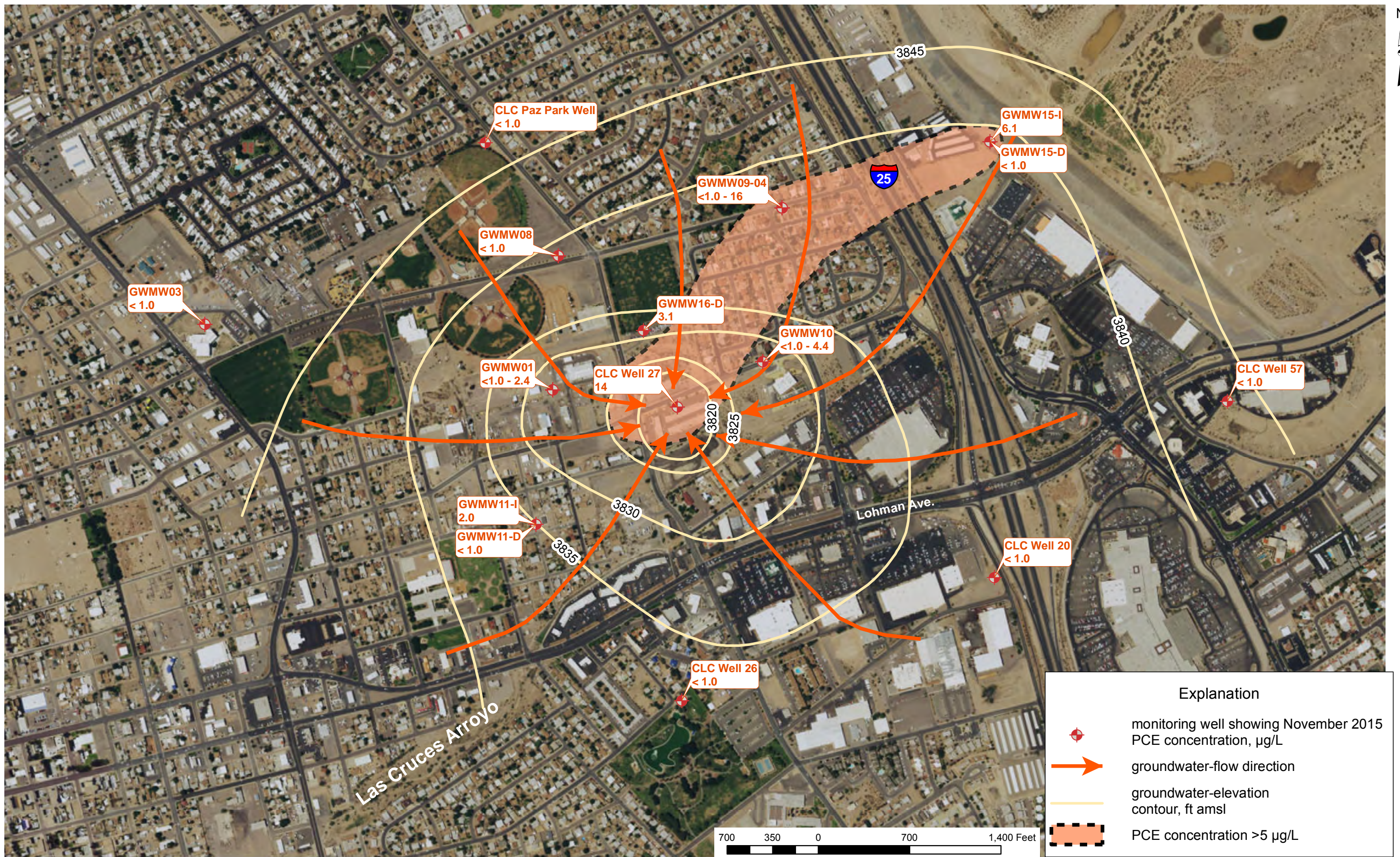
Figure 9. Aerial photograph showing November 2015 PCE concentrations and groundwater-elevation contours for the Lower Hydrogeologic Zone, Griggs and Walnut site, City of Las Cruces, New Mexico.
