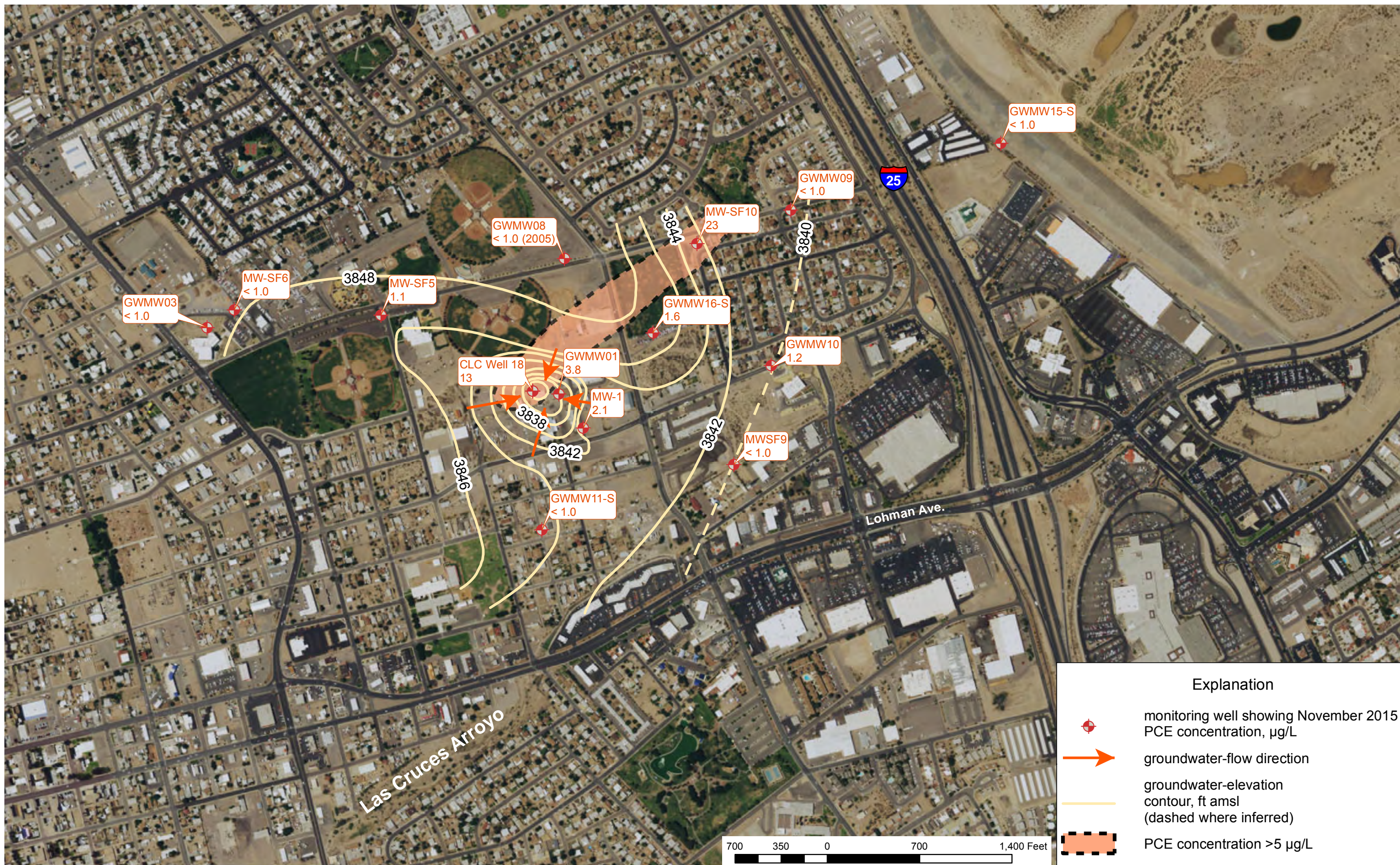
Figure 8. Aerial photograph showing November 2015 PCE concentrations and groundwater-elevation contours for the Upper Hydrogeologic Zone, Griggs and Walnut site, City of Las Cruces, New Mexico.
